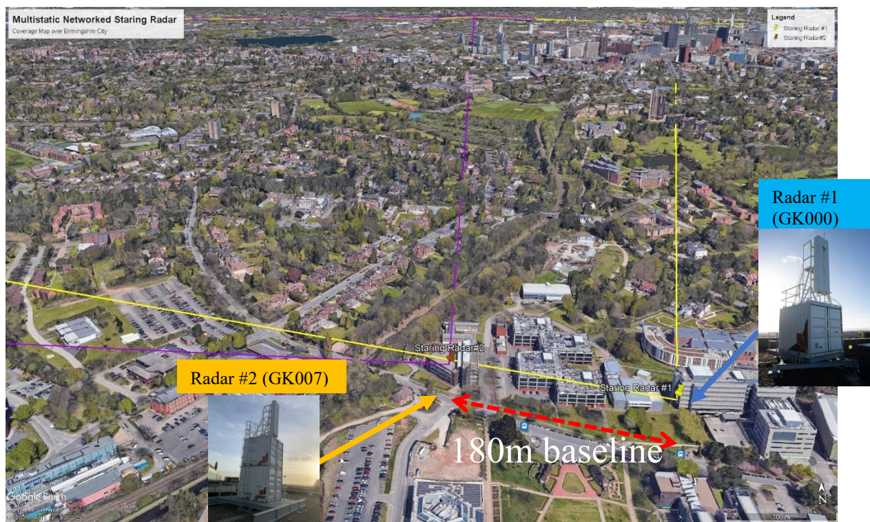
Figure 3: Coverage map for Radar #1 (yellow) and Radar #2 (purple). Bistatic baseline is 180m.
