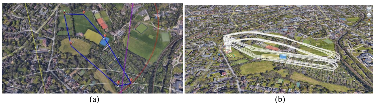
Figure 4: (a) Flight path waypoints plotted as blue lines (b) Drone GPS truth plotted as white lines showing data from multiple flights at two heights
